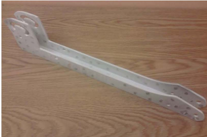
Figure 3.1. Bracket support part from a manual powered scooter.
