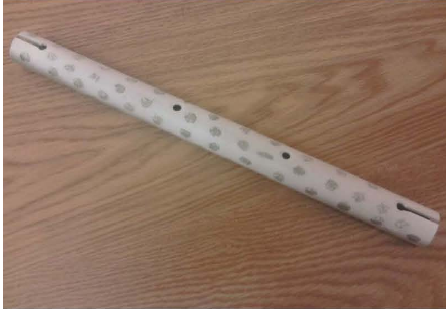
Figure 3.2. Pipe support part for the handlebars of a manual powered scooter.
